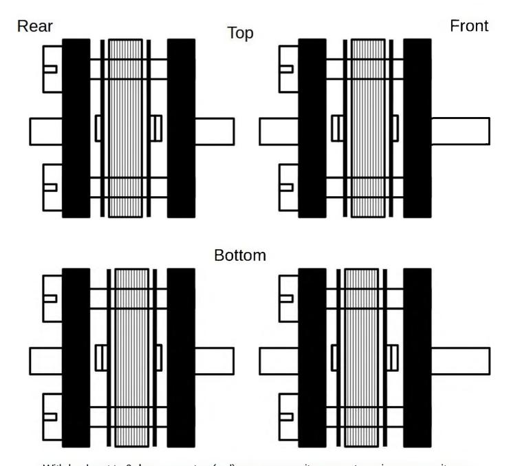
With knob set to 0 degrees on top (red) cursor, capacitors are at maximum capacitance.
